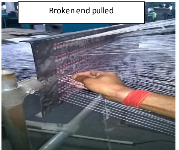
End passed from leasing comb
