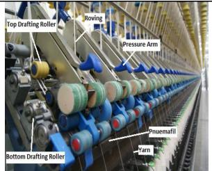
**Twisting:** The drafted strand of the material is finer than rove and twist is inserted to strengthen the material i.e. yarn.
